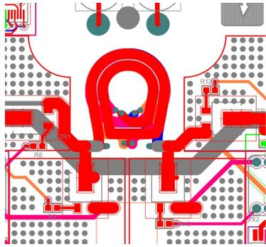
Irregular spiral shapes can be created using the Pulsonix Embedded Component option defining the footprint as embedded, the Component can be mirrored in situ and all the inner layers will swap as required. Special DRC properties also allow the checking of correct internal connectivity made on the elements of these components.
