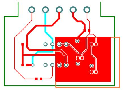
Now when you use **Pour Copper** from the context menu for the selected Template, the area will be flooded with copper that has thermal connections and isolation gaps on the 0V nets.
