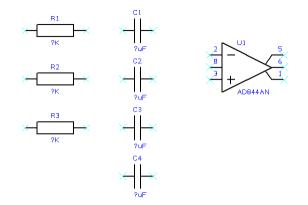
Before we make the connections we should change the **Component values** to be the ones required. This is easy to do because we've used 'generic' resistor and Capacitor components.
