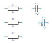
Move C2 away and just underneath C1 by moving the mouse and single click to release. Now do the same again to **C2** to add another capacitor **C3** and then again with **C3** to add **C4**.
