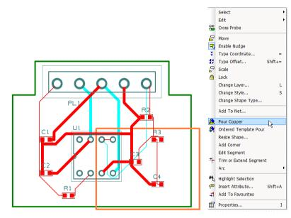
The template will fill with copper. Notice that the poured copper has obeyed the Technology **Spacing** rules of all defined items to copper, including the Board to Copper rules.
