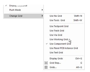
By default, the Component grid has been set fairly coarsely at 100 Thou and the Working grid set finer at 25 Thou. These can both be changed (as can all the system grids).
