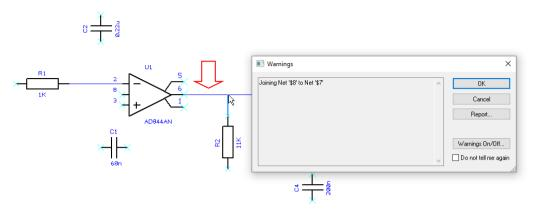
In the example above, this dialog warns you that the net \$8 is about to be connected to the existing \$7 and renamed. Yours may show slightly different net names. The \$ names are automatic net names created by the system and can be renamed at any time anyway.
