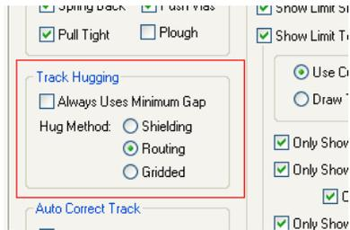
**Shielding** adds tracks that hug the obstacles as tight as possible, introducing arcs around pads and sharp corners (see below). This can be used to create shielding around tracks and other copper obstacles for RF protection for example.
