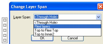
Components which are to be used on any other layer span other than conventional <Through Hole> do not need any special set up requirements but you should be aware of any supporting layers which may or may not be subsequently required, for example Silkscreen layers.
