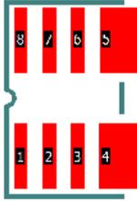
*Note that when designing multiple footprints to represent the different arrangement of thieving pads all other aspects of the footprint, including its orientation, should remain constant across all the footprints, only the position and size of the thieving pads should vary.*
