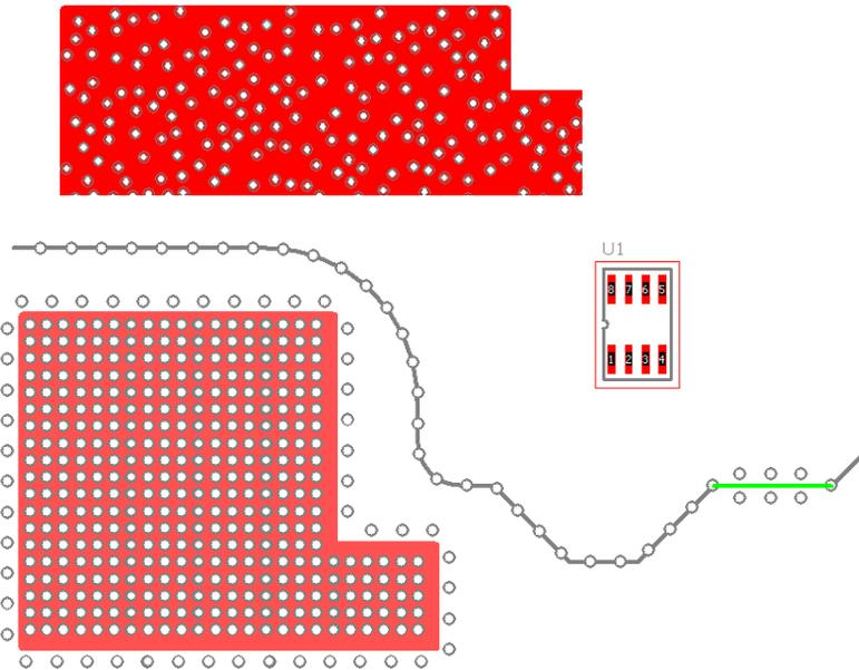
Using the **Around Inside** option, vias could be placed inside a board outline, like the example below:
