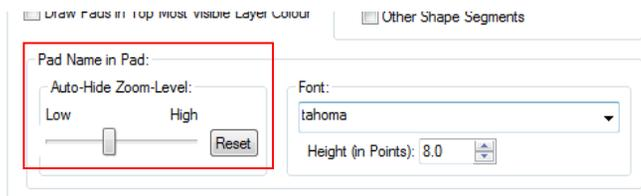
Setting the slider to a **higher** position avoids situations like this below where the pads can't be seen under the pad names:
