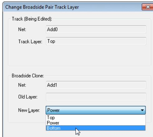
For Broadside coupling the paired length will be calculated where one track is completely over the other, but if both edge and broadside coupling is allowed, both types of paired sections will be added together to give the total figure.
