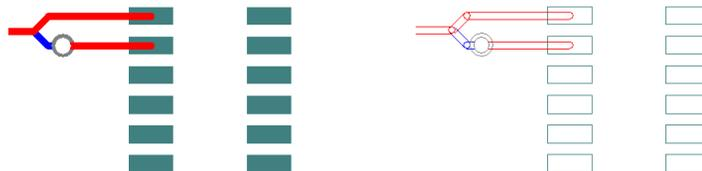
The above example shows the design before and after the **Toggle True Width** commands have been used.
