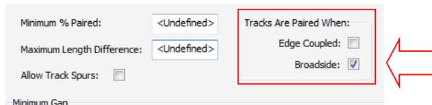
For **Broadside** only coupling, the gap can still be provided and will be used for the minimum separation of the tracks when they are on the same layer, for example when routing out of surface mounted pads but this will not contribute to the % paired.
