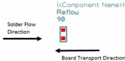
The Footprint Rules dialog could look like the example below. The rules dialog does not need to have the <Orientations> attribute defined here, it will be automatically matched using the Flow Direction defined in the rule.
