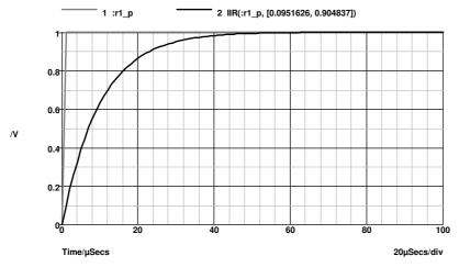
The coefficients used give a time constant of 10 \* the sample interval. In the above the sample interval was 1µSec so giving a 10µSec time constant. As can be seen a first order IIR filter has exactly the same response as an single pole RC network. A general first order function is:
